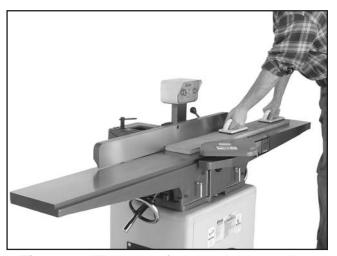
Figure 22. Typical surface planing operation.
